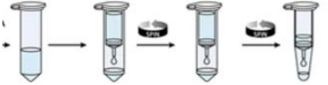
Add ethanol and mix Add sample to spin cartridge Wash Elute RNA with RNase-free water
